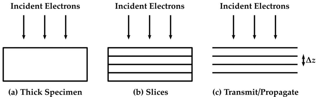
**FIG. 10.** Diagrams showing (a) the full specimen, (b) the specimen separated into thin slices, and (c) how each slice involves transmission through a slice, followed by propagation through vacuum of thickness  $\Delta z$ .
