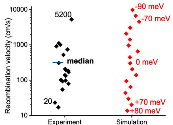
FIG. 21. Experimental recombination velocities from Ref. 51 and simulated values using Eq. (4). The median value of about 300 cm/s is highlighted by a horizontal, solid line and used as  $s_{gb,0}$  in Eq. (4). The barrier heights obtained from Eq. (4) are given in red next to the simulated recombination velocities.
