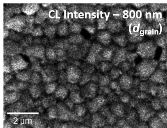
FIG. 22. CL intensity distribution acquired on a Cs<sub>0.05</sub>(FA<sub>0.95</sub>MA<sub>0.05</sub>)<sub>0.95</sub>Pb(I<sub>0.95</sub>Br<sub>0.05</sub>)<sub>3</sub> thin film using a bandpass filter at 800 nm ( $\pm 50$  nm), corresponding to the bandgap energy of the halide-perovskite thin films of about 1.54 eV. Reproduced with permission from Gutierrez-Partida *et al.*, ACS Energy Lett. 6, 1045–1054 (2021). Copyright 2021 American Chemical Society.<sup>260</sup>
