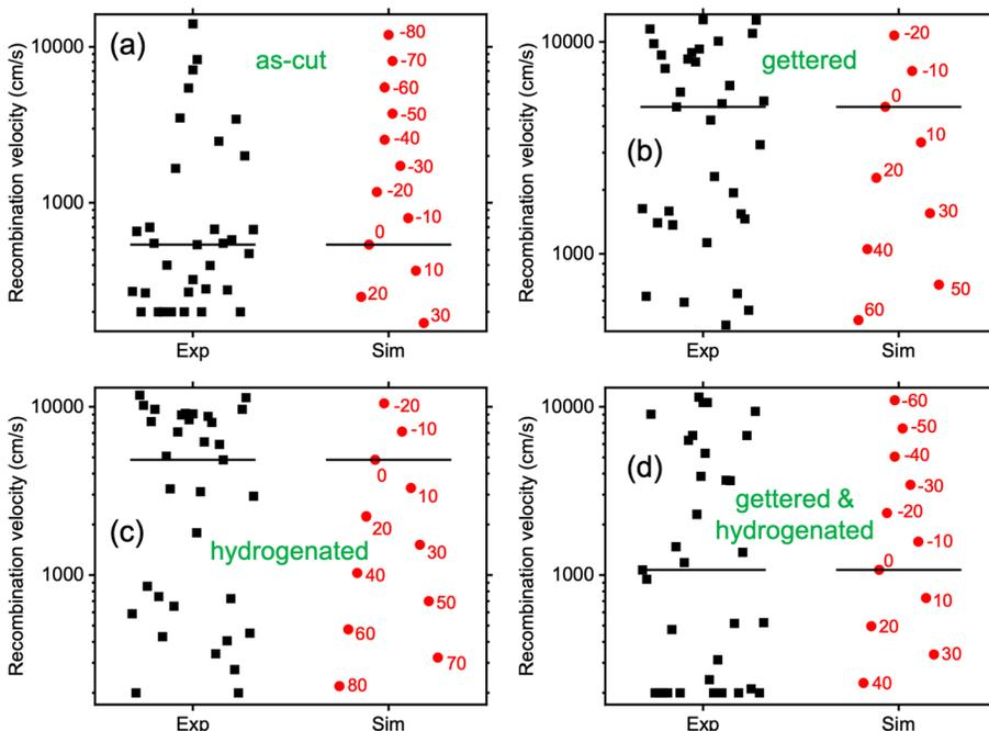
**FIG. 20.** Experimental (Exp) recombination velocities from Ref. 231 (*p*-type mc-Si) and simulated (Sim) values using Eq. (4). The median value for each sample series is highlighted by a horizontal, solid line and used as  $s_{gb,0}$  in Eq. (4). The barrier heights obtained from Eq. (4) are given in red next to the simulated recombination velocities.
