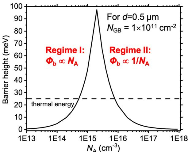
**FIG. 4.** Barrier at the grain boundary as a function of the net-doping density  $N_A$ . The assumed average grain size  $d_{\text{grain}}$  and (charged) defect density  $N_{gb}$  at the grain boundary plane were  $0.5 \mu\text{m}$  and  $1 \times 10^{11} \text{ cm}^{-2}$ , respectively. The thermal energy at room temperature,  $k_B T \approx 25 \text{ meV}$ , is indicated by a horizontal, dashed line.
