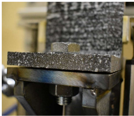
(b) Gap caused by flange bowing
