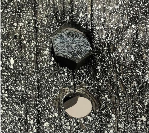
(b) Shear-out failure
