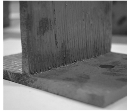
(a) Sharp corners, flanges and web continuously printed
