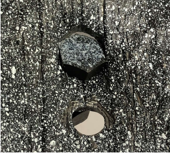
(c) Punching failure (Specimen T2-140-1.83-C-R)
