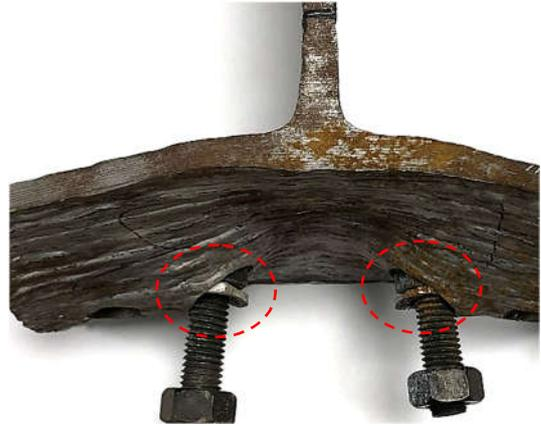
(c) Punching failure (Specimen T2-140-1.83-C-R)
