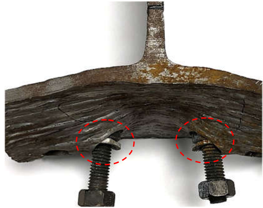
(c) Punching failure (Specimen T2-140-1.83-C-R)
