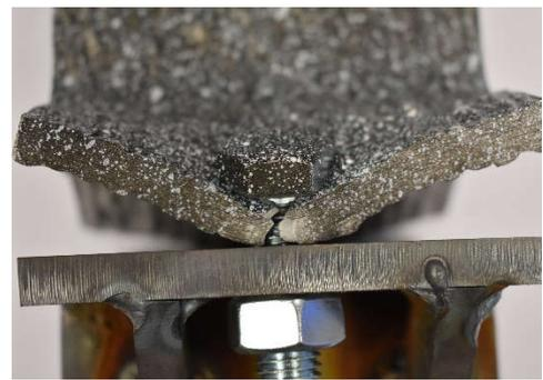
(a) Ultimate bolt failures
