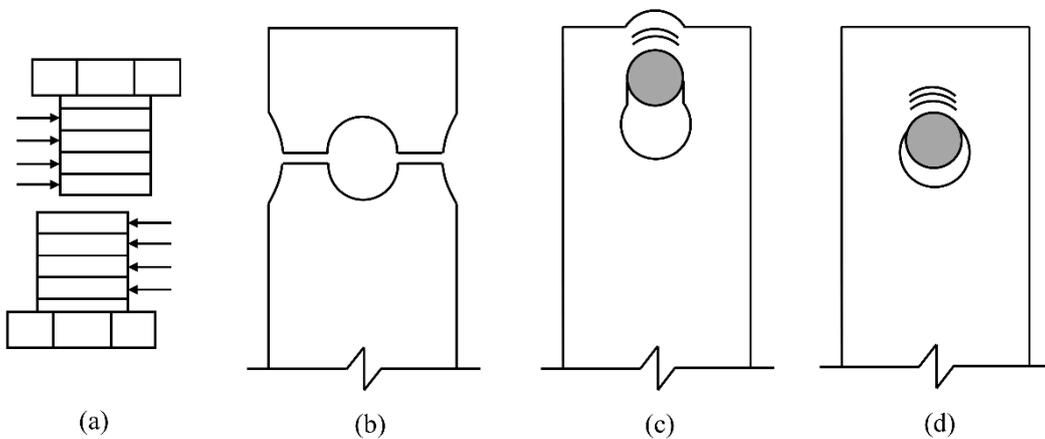
79 Figure 1. Schematic representation of failure modes: (a) bolt shearing, (b) net section tension, (c) shear-
