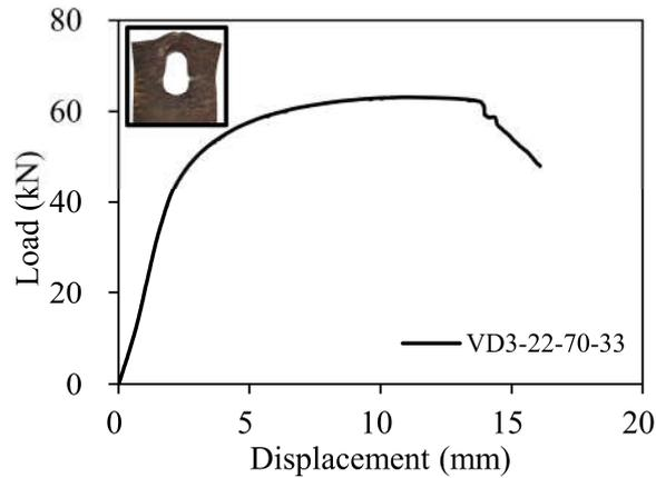
Figure 8. The load-displacement curve of VD3-22-70-33 failing by block shear
