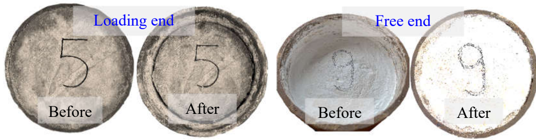
(a) Loading and free ends of the specimens before and after the test
