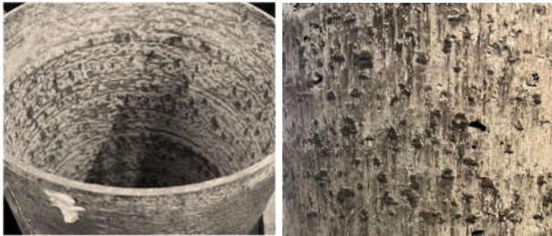
(b) Typical interfacial surfaces of tube and concrete after push-out test
