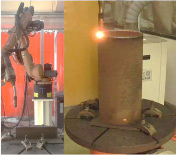
(a) Printing of a subset of the WAAM CHS steel tubes
