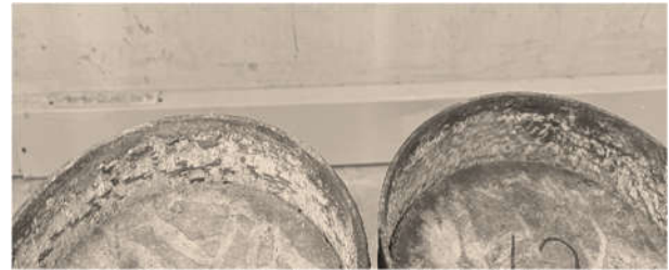
(c) Comparison of loading ends with different tube thickness
