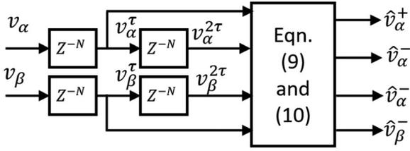
FIGURE 2 Proposed arbitrarily fast modified DSC method
