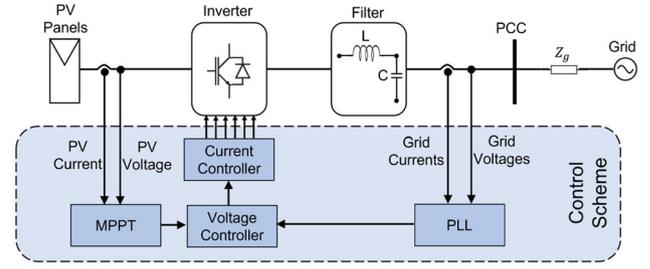
**FIGURE 1** An overview of a general grid-connected converter control system with PLL-based grid-synchronization method
