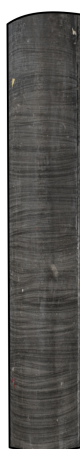
Video. 1. Photogrammetric model of an internal levée core section (BAV 2, 73.07–73.45 m, core width: 65 mm). Model highlights the three-dimensional geometry and texture of small-scale hummock-like and swale-like laminasets (HLCS), and their gradual transition from swale-like to hummock-like within laminasets.
