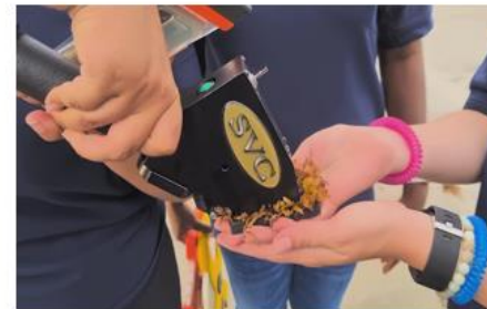
Field spectrometer (SVC HR-1024i) data collection Method 2 (Ghana)
