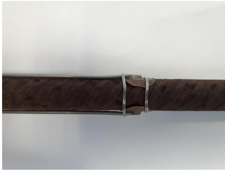
Figure 1: Example of thermocouple installation for rebar temperature measurements
