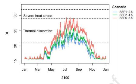
Figure 4. Time course of the discomfort index (DI) in the test house in 2100 (hourly means)under different SSP scenarios.
