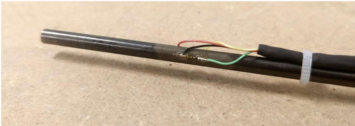
Figure 3: MaCE pressure bar. High strain capacity semiconductor gauges are bonded to a 4mm diameter maraging steel bar, 40mm from the loaded face.
