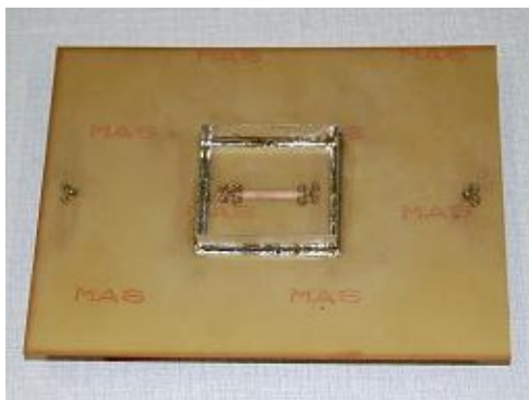
a) with shield lid removed showing stripline
