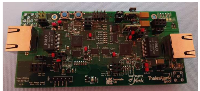
Fig. 6. Prototype SpacePHYre PCB supporting two Microchip VSC8541 PHYs (the commercial equivalent part of the VSC8541RT) and matched magnetics, the board is plugged in to an Ultra96 FPGA board where the CODEC is implemented within the FPGA hardware.
