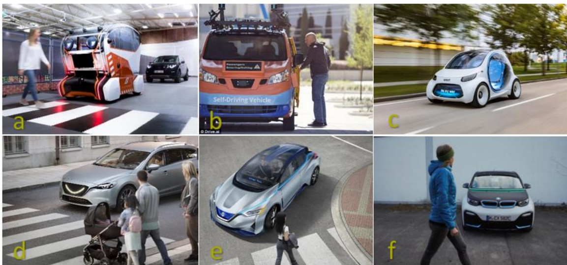
71 72 Figure 1: Example of eHMI concepts from (a) Jaguar Land Rover , (b) Drive AI , (c) Mercedes Benz , (d) Semcon , (e) Nissan 73 Motor Corporation , and (f) interACT project
