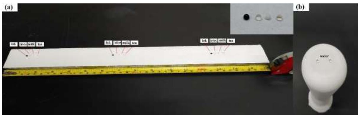
494 **Figure. 14.** Digital photos of the large scale&irregular shape samples with 2.5EPZF coating and their
