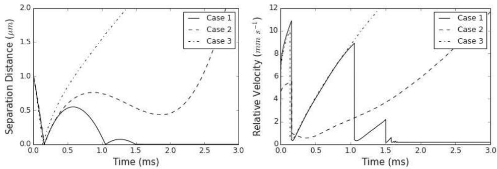
Figure 2: Temporal evolution of separation distance and relative velocity of three illustrative interaction cases between disks.
