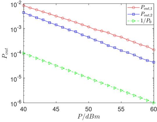
Fig. 7. Outage probabilities at a high SNR condition.
