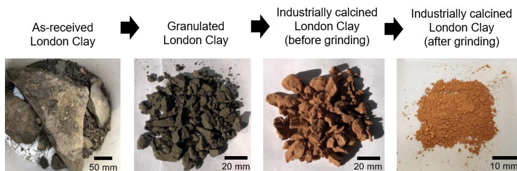
216 217 Figure 2: Photographs of the Westgate clay at various stages of the industrial calcination 218 process, with approximate scale bars to indicate changes in feed and particle size.
