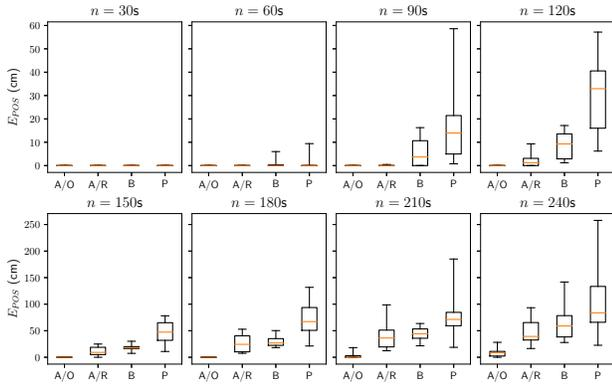
Fig. 4.  $E_{POS}$  after  $n$  seconds for simulated nodes using the AirTight protocol with optimal (A/O) and randomised (A/R) routing, Broadcast protocol (B), and Point-to-point protocol (P) over 10 different random seeds. Note that the y-axis scaling changes between rows.
