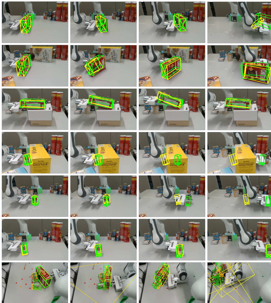
Fig. 2. Experimental Scenes. The images are from the tracking camera. The estimated object pose of our method (PBPF) is shown as a green wireframe box, while the estimated object pose from DOPE is shown as a yellow wireframe box.
