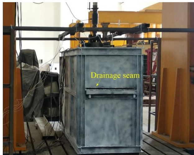
Fig. 7 The photograph of the test model (with rainfall simulator uninstalled)
