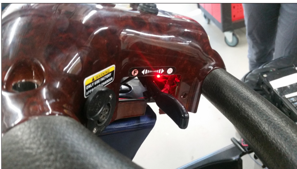
Figure 12 Steering console showing the newly added relay (with lit LED).
