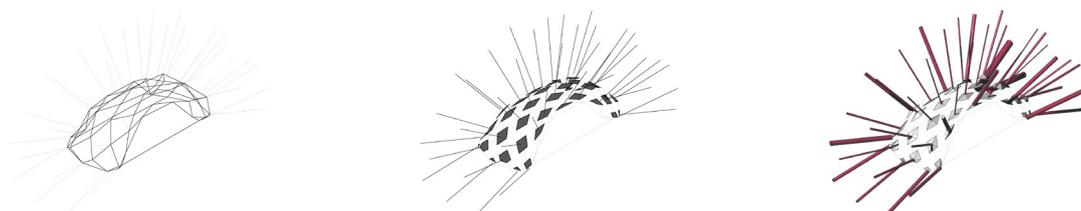
Fig.7: Introducing the Doo-Sabin mesh subdivision for determining force, the areas of the polygonal geometries created are assumed to provide the amount of force for each wire in tension; pipe diameters graphically show the deviation from OasysGSA values.
