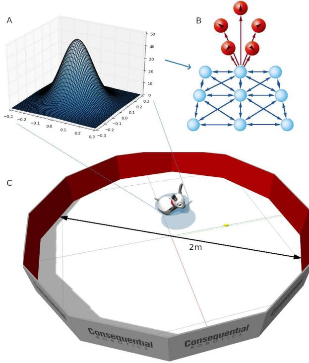
Fig. 4: Hippocampal striatal network. A. Each place field is a Gaussian centered at a given preferred position. B. The network is composed of the hippocampal network that has a feed-forward projection to action cells. C. The simulations are performed in a circular arena with the robotic platform MiRo-e.
