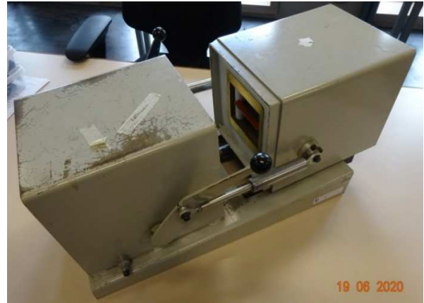
Fig. 7. Far-field TEM-t fixture.
