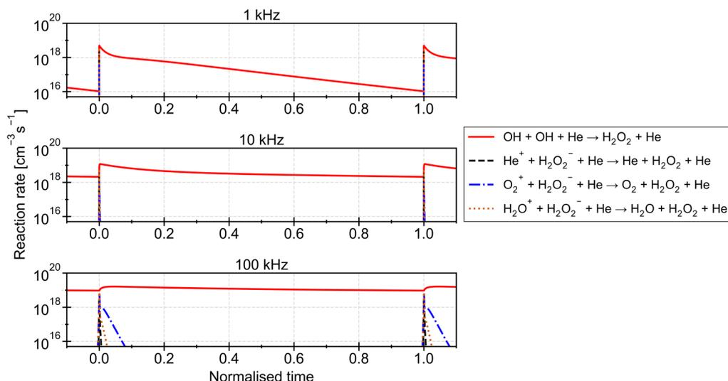
FIG. 11. Rates of dominant H<sub>2</sub>O<sub>2</sub> production reactions over one cycle for 1, 10, and 100 kHz pulse repetition frequencies.
