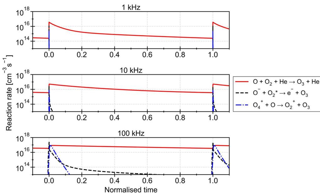
FIG. 16. Rates of dominant O<sub>3</sub> production reactions over one cycle for 1, 10, and 100 kHz pulse repetition frequencies.
