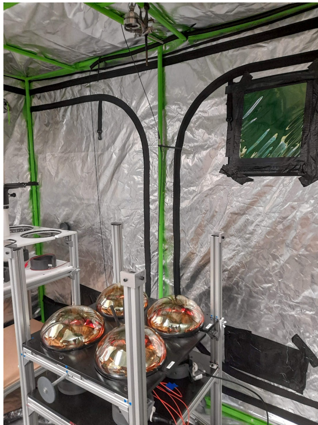
Figure 2. Mounting of the PMTs in the mechanical rig in the tent. Optical fibres guide the light from the LED box outside the tent to the diffuser, which hangs from a fixation point on the tent roof at the top centre of the image.
