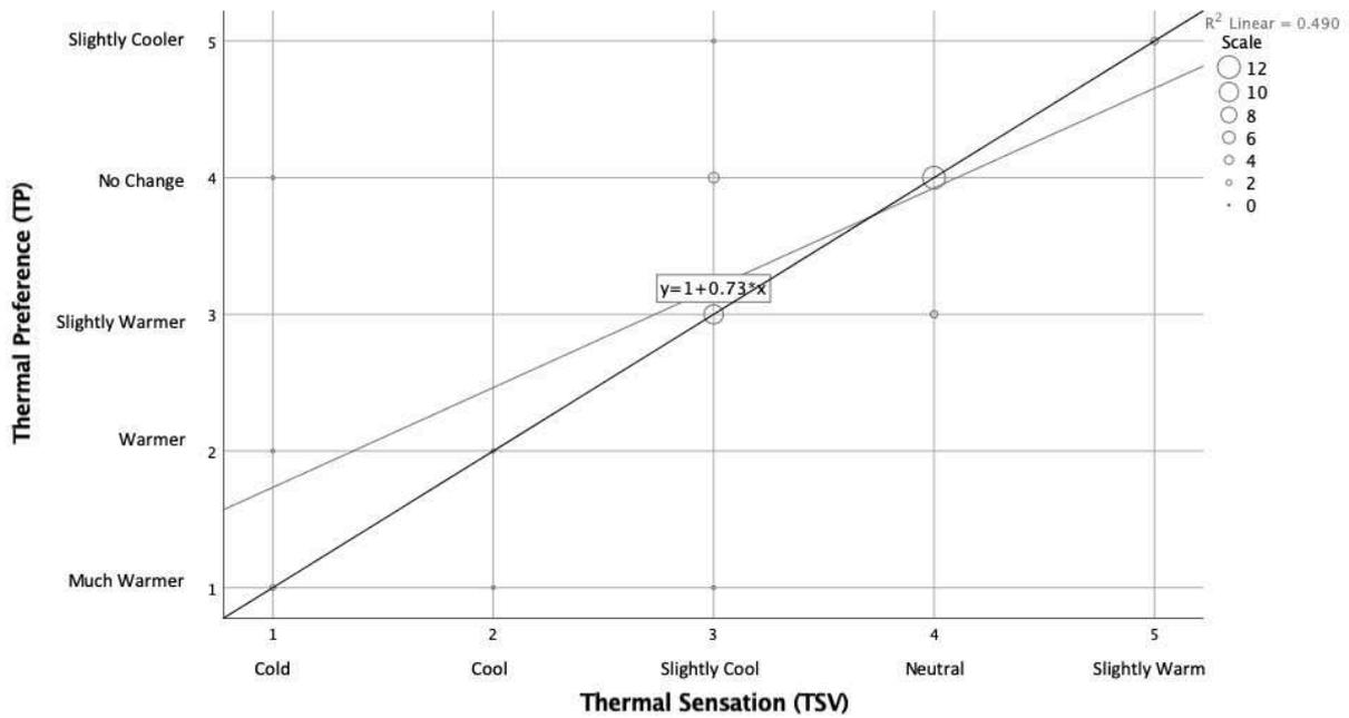
Figure 12. The relationship between thermal sensation and thermal preference
