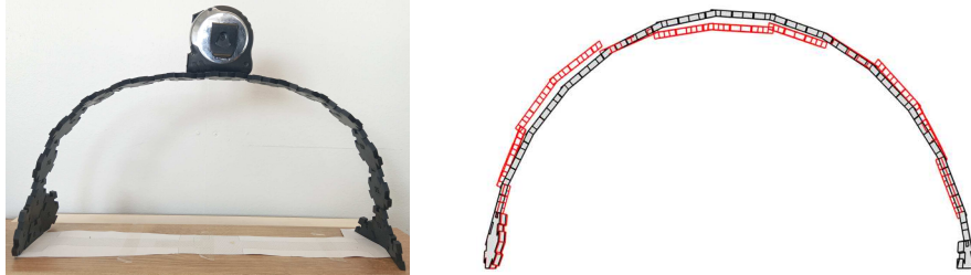
Fig. 5: Dead load testing. Left) The shape of the structure can be seen with a mass on the central panel. Right) The CRA model of the structure with its ultimate load, where the panels are predicted to separate (original design in black, failure mode in red).
