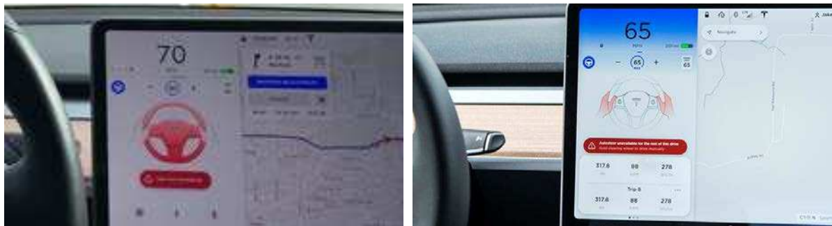
Figure 4: Left: Tesla's take-over request due to a technical limitation/failure. Right: Tesla's hands-on request after the driver kept their hands off for too long.
