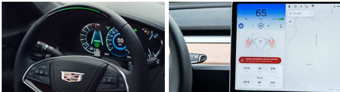
Figure 6: Left: Cadillac's LED strip used to indicate system status and warn drivers with flashing red lights. Right: Tesla's centre console flashing blue to warn drivers.
