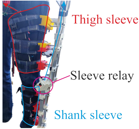
Fig. 3. Test subject in sensing sleeve and exoskeleton with covered sleeve areas highlighted
