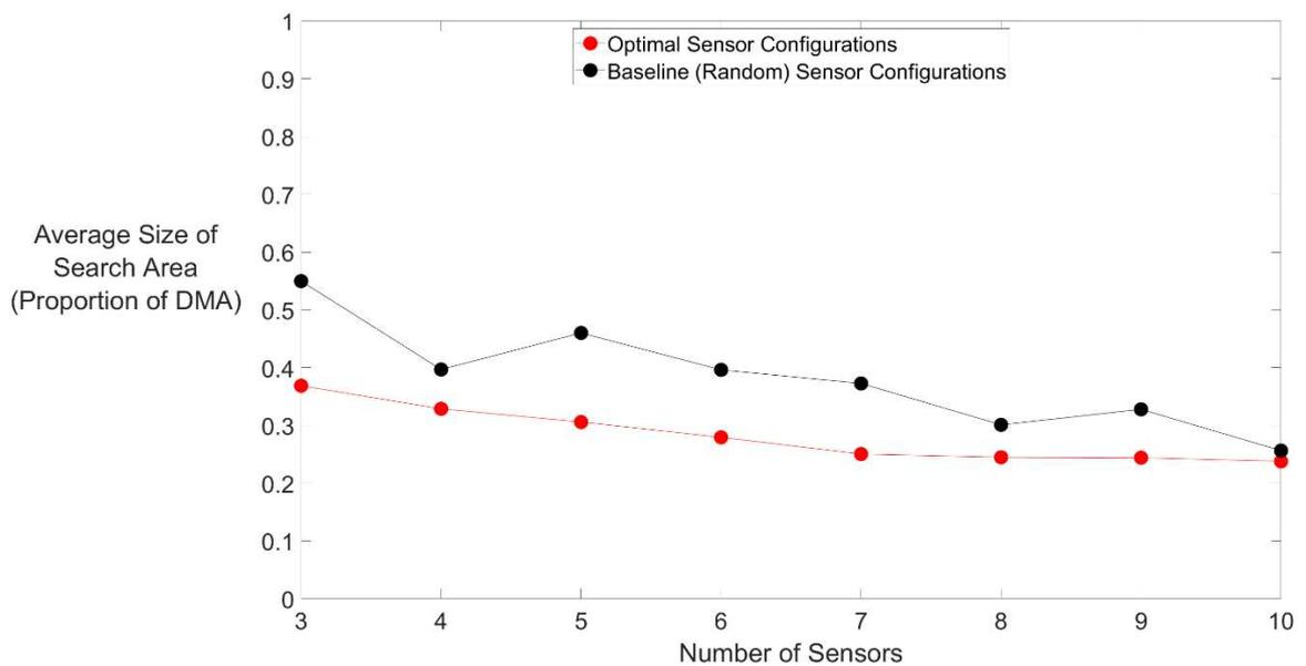
520 **Figure 4:** Comparison of the performance for the constrained optimal and baseline sensor
