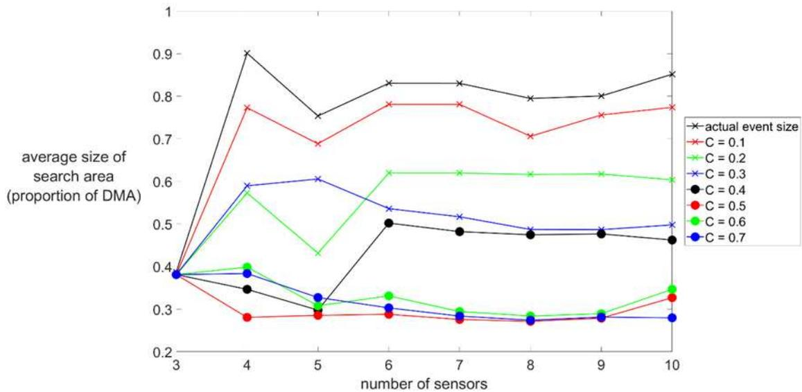
673 **Figure 9:** Comparison of the leak/burst localisation performance for 16 modelled events
