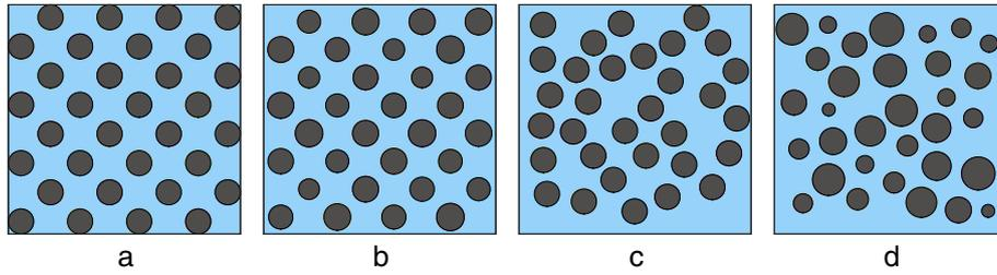
**Fig. 2** Example of test materials. Periodic (a), randomness in particle size (b), position (c) and both (d). ( $V_f = 30\%$ )
