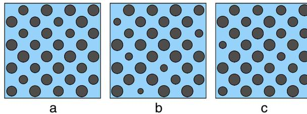
**Fig. 8** Randomness added to particles sizes. Three different realisations a, b and c from left to right. ( $V_f = 30\%$ )
