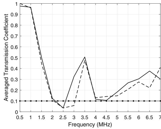
**Fig. 3** The average transmission coefficient  $\bar{T}$  and effect of magneto-elastic coupling on the stop-band frequencies in periodic microstructure. Decoupled (solid), coupled (dashed) of magnetic field cases. Dashed-dotted line presents 10% cut-off indicating stop-band
