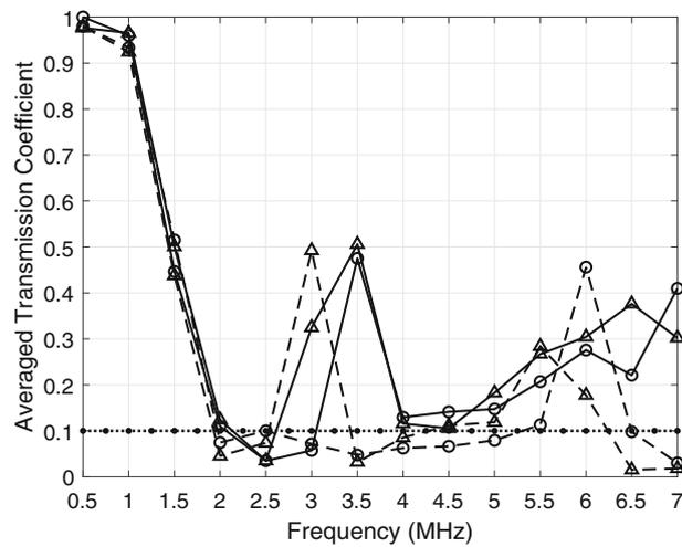
**Fig. 5** The average transmission coefficient  $\bar{T}$  and the effect of volume fraction on the wave propagation in coupled (circle)/decoupled (triangle) cases.  $V_f = 30\%$  (solid) and  $V_f = 45\%$  (dashed)
