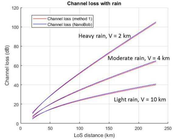
Fig. 5 Channel loss with the presence of rain
