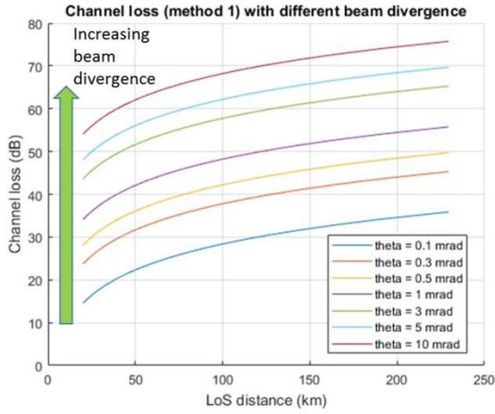
Fig. 8 Channel loss with varying beam divergence
