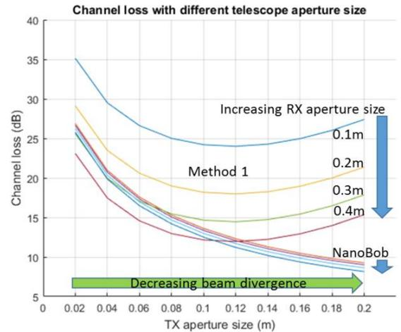
Fig. 7 Channel loss with varying telescope aperture size
