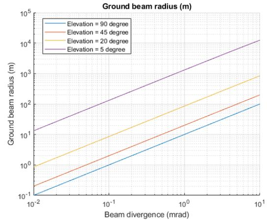
Fig. 11 Ground footprint size against beam divergence
