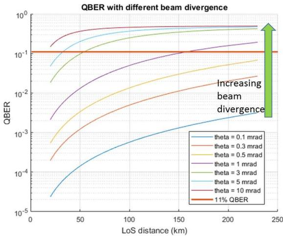
Fig. 9 QBER with varying beam divergence for DV-QKD
