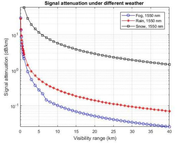
Fig. 2 Optical signal attenuation under different weather conditions
