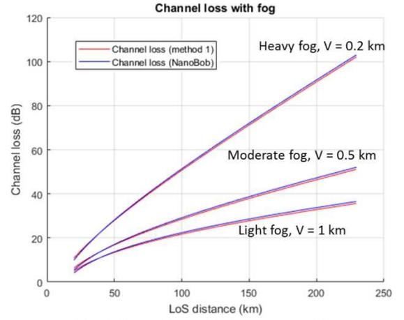
Fig. 4 Channel loss with the presence of fog
