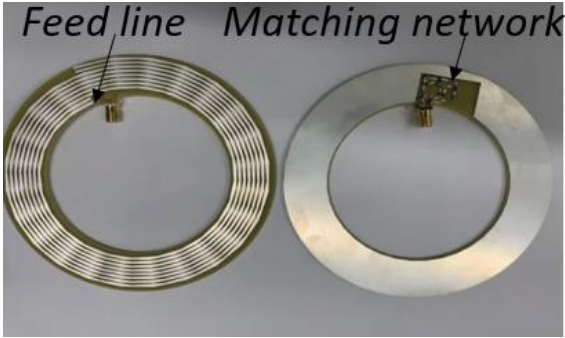
Fig. 6. A fabricated prototype of MASA.
