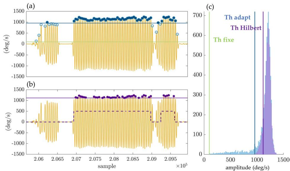
**Fig. 4** Thresholding methods for peak selection, example based on data from one subject: **(a)** the filtered signal  $\omega N$ -LPF-CWT (orange) is shown, as well as the obtained  $TH_{adapt}$  (dark blue) and the selected peaks (dark blue starts with amplitudes above the thresholds); **(b)** the Hilbert envelope method is shown with the preselected walking periods (dashed line), and the selected peaks (dark purple dots); **(c)**
