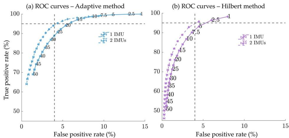
**Fig. 6** ROC curves for performance evaluation as a function of percentile values from 1 to 50% when the angular velocity norm  $\omega N$  is used as input. The curves are obtained by averaging the results over the 10 subjects when one IMU (continuous line) or two IMUs (dashed line) are used; **(a)** Adaptive threshold method ( $TH_{adapt}$ ) based on the percentile of the obtained peak amplitude distribution
