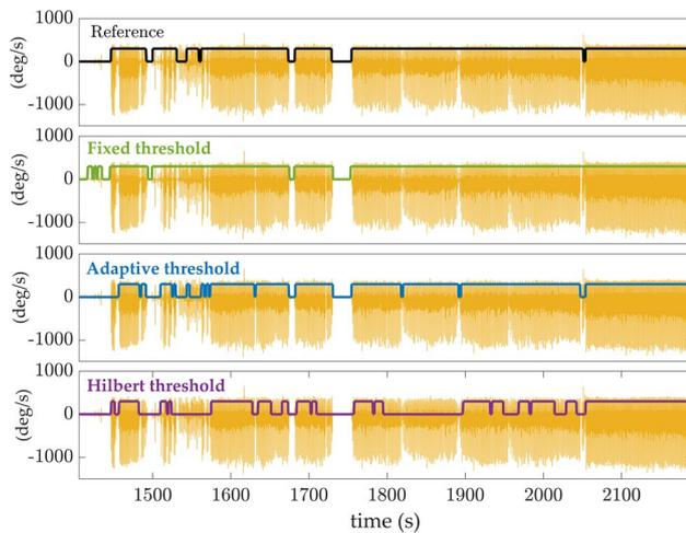
**Fig. 5** Illustration of walking detection using the different thresholding methods on data recorded in one subject: *fixed* threshold (green), *adaptive* threshold (blue) and *Hilbert* threshold (purple). The reference classification, obtained from the plantar pressure of the INDIP system, is displayed in black at the top of the figure
