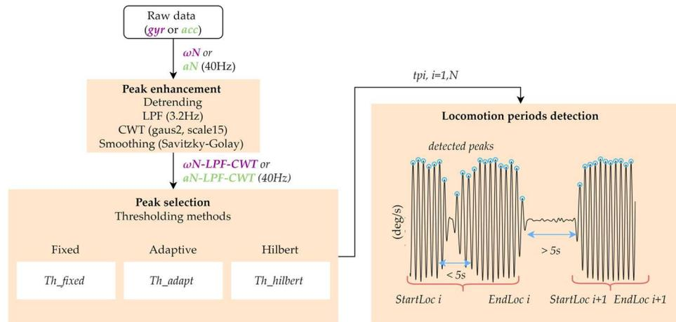
**Fig. 2** Flowchart of the walking bouts detection algorithm for one-foot IMU.  $\omega N$ : raw angular velocity norm;  $aN$ : raw acceleration norm; LPF: low-pass filter; CWT: continuous wavelet transform;  $TH_{fixed}$ : fixed threshold ( $TH_{fixed} = 100\text{deg/s}$  or  $TH_{fixed} = 0.5\text{g}$ );  $TH_{adapt}$ : adaptive threshold based on the percentile of the obtained
