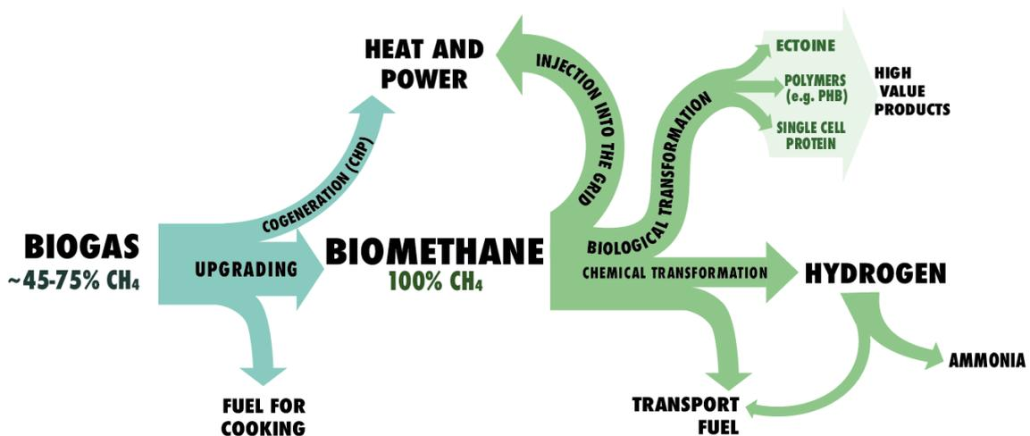
**Figure 3: Potential biogas applications.** Biogas and upgraded biomethane is currently mainly consumed as a fuel for heat, power and cooking (blue), but could be
