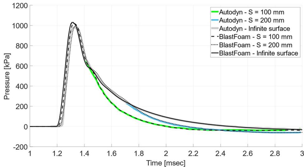
**Figure 5. Comparison of free-air explosion ( $Z = 1.6 \text{ m/kg}^{1/3}$ ) pressure-time histories derived from BlastFoam with digitised values from Autodyn (Shin and Whittaker 2019) for an infinite surface and finite surfaces of half widths of  $S = 100 \text{ mm}$  and  $200 \text{ mm}$ .**
