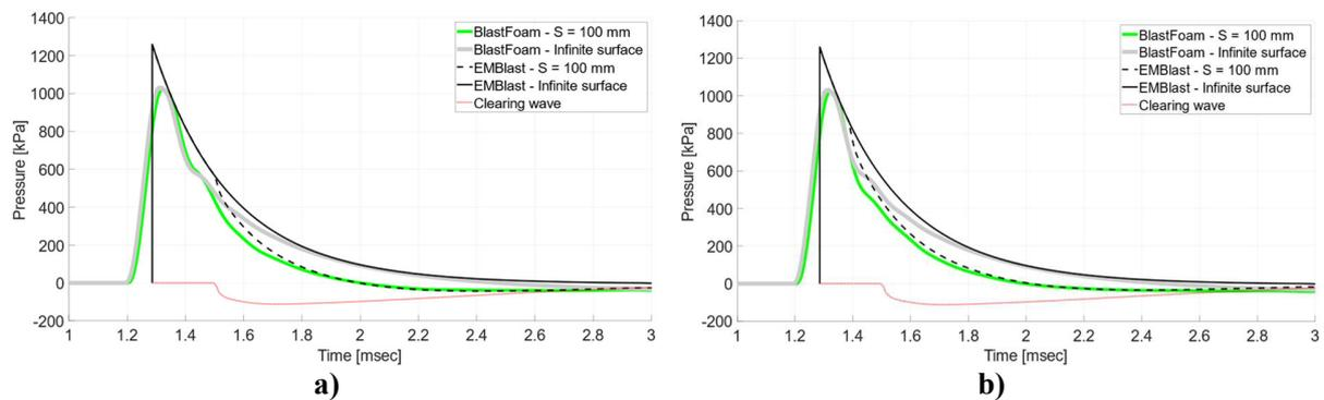
**Figure 6. Comparison of the pressure-time histories derived with EMBlast and BlastFoam for a free-air explosion ( $Z = 1.6$  m/kg<sup>1/3</sup>) for a finite size target of half-width  $S = 100$  mm: a) 100 mm away from the free edge, b) 50 mm away from the free edge.**
