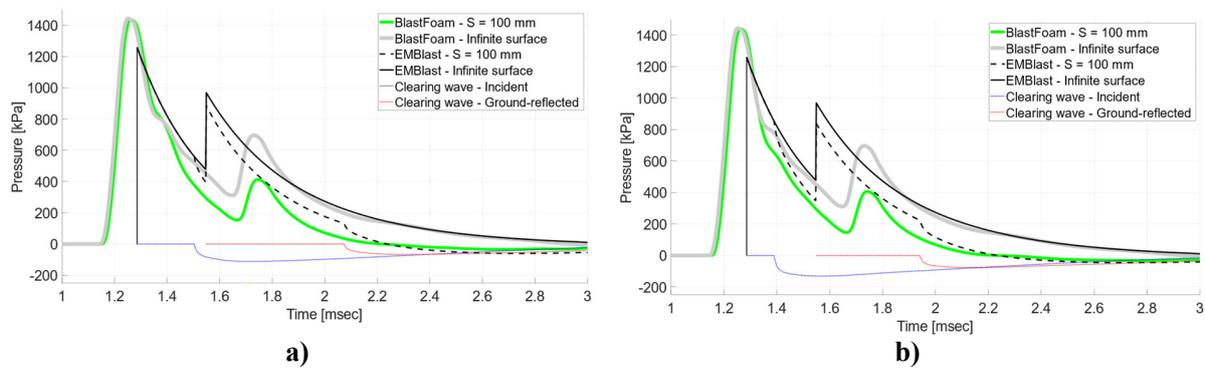
**Figure 7. Comparison of the pressure-time histories derived with EMBlast and BlastFoam for an above-ground explosion ( $Z = 1.6 \text{ m/kg}^{1/3}$ ,  $V_E = 0.6 \text{ m}$  and  $V_T = 0.6 \text{ m}$ ) for a finite size target of half-width  $S = 100\text{mm}$ : a) 100mm away from the free edge, b) 50mm away from the free edge.**
