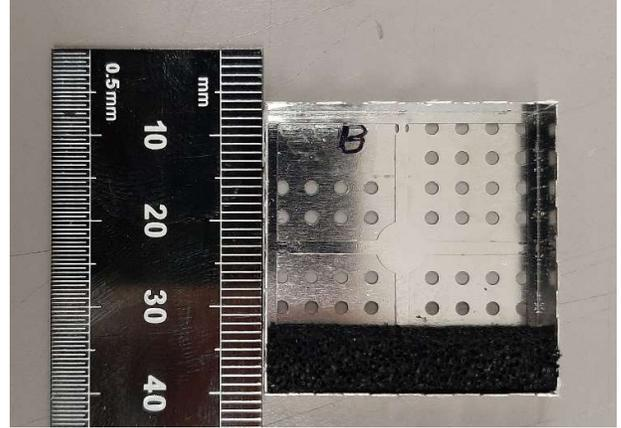
Fig. 3. LS22 absorber block installed in the PCBS.
