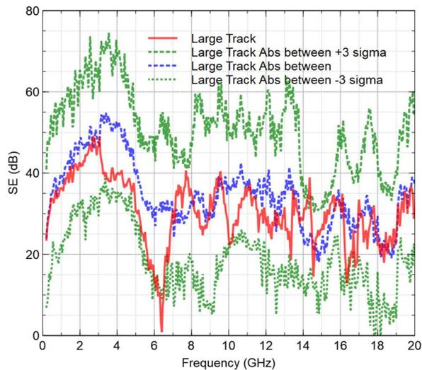
Fig. 12. Comparing *SE* for the jig with absorber between the shield stripline in the PCBS and the external stripline with no absorber in the PCBS with a  $50\Omega$  load on the shield stripline in both cases
