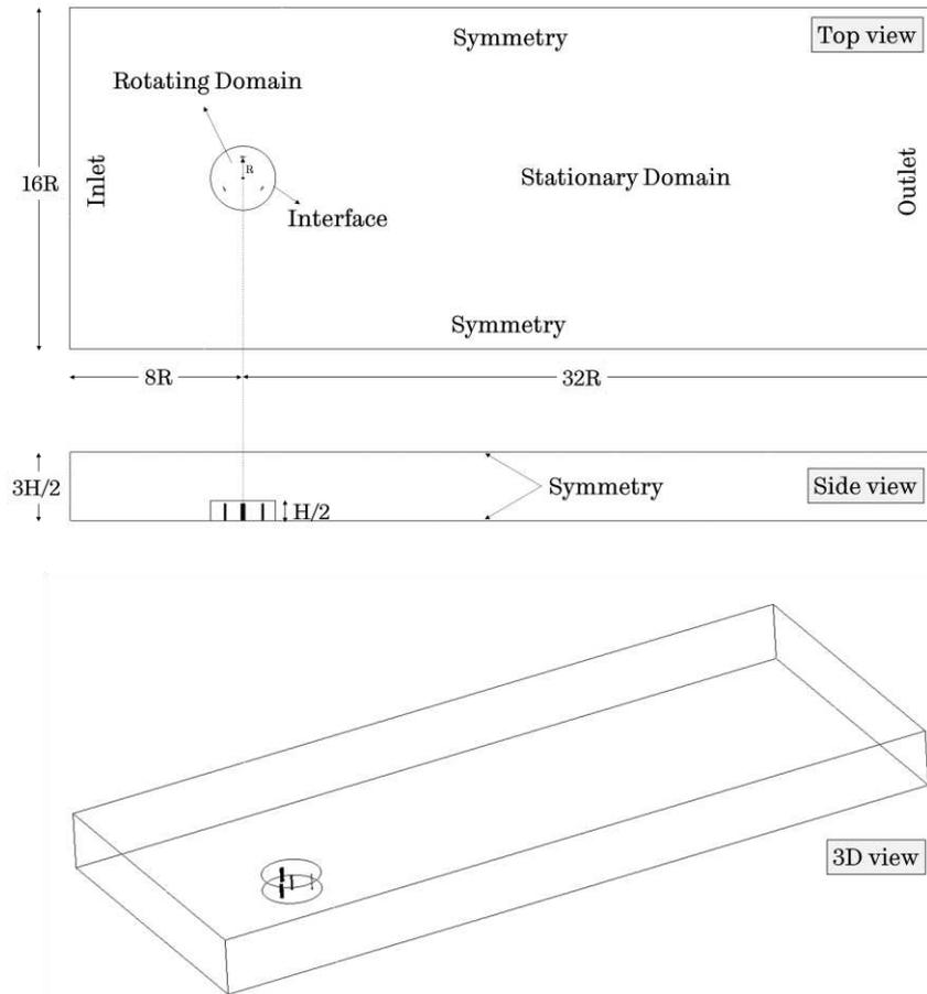
Fig. 2. Three-dimensional computational domain used in the present CFD calculations and the boundary conditions.
