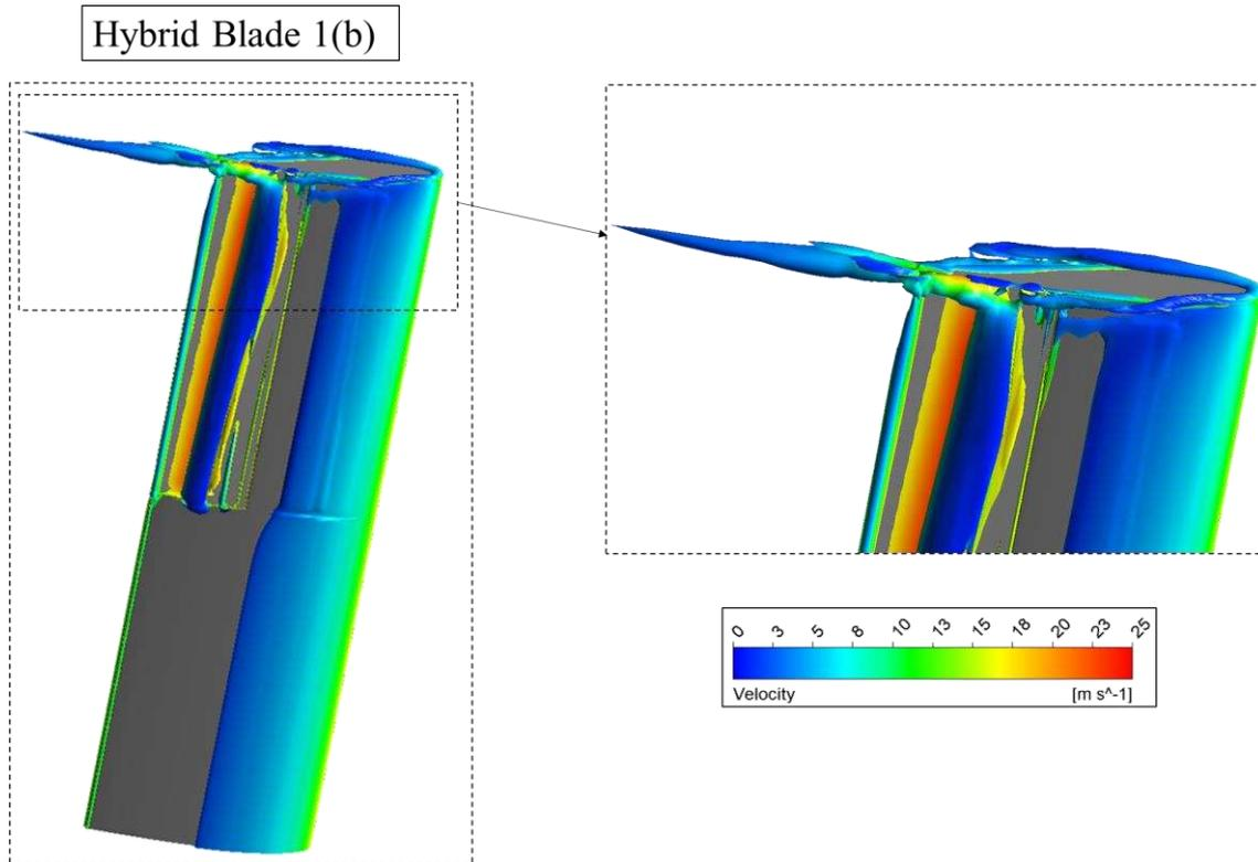
Fig. 12. The iso-surface contours for the vortex structures generated around the turbine with the Hybrid Blade 1(b) configuration with an enlarged view of the blade tip at  $\lambda=2.25$ .
