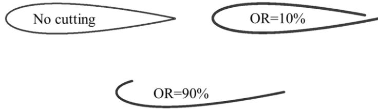
Fig. 8. The schematic of the airfoils with and without openings (OR: Opening Ratio over the J-shaped airfoil).
