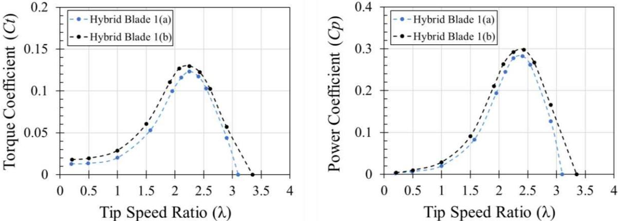
Fig. 16. The comparison of the torque and power coefficients of the turbines with the Hybrid Blade 1(a) and Hybrid Blade 1(b) at various tip speed ratios.
