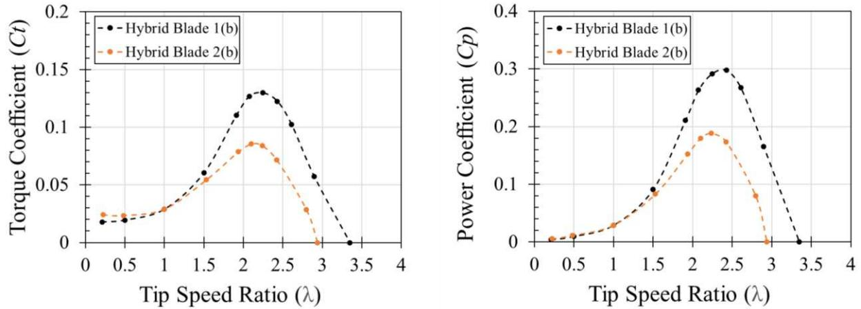
Fig. 17. The comparison of the torque and power coefficients of the turbines with the Hybrid Blade 1(b) and Hybrid Blade 2(b) at various tip speed ratios.
