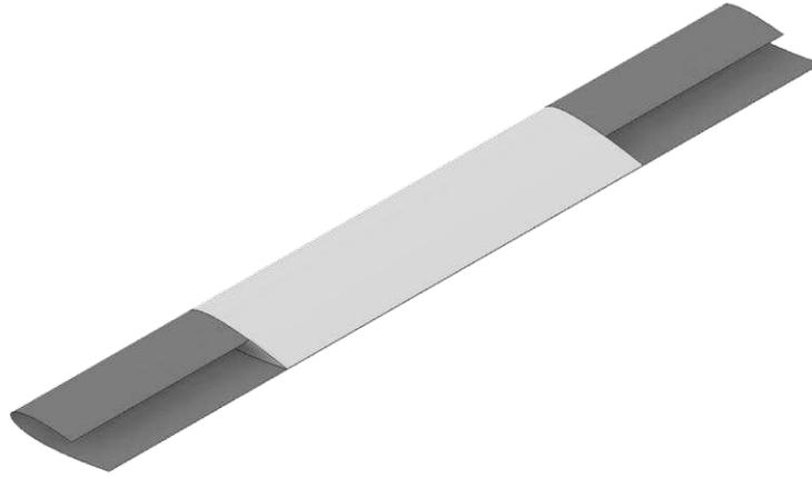
Fig. 1. Schematic of the one of the proposed Hybrid Blade designs having a conventional NACA0018 airfoil and its 40% opening J-shaped profile.
