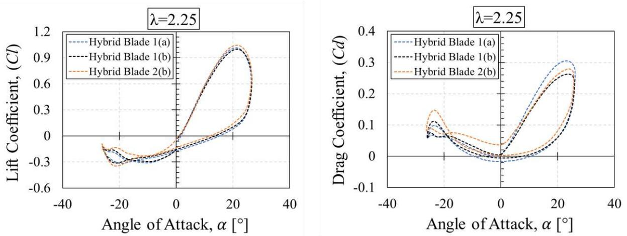
Fig. 19. Comparison of the lift coefficient and drag coefficient between the hybrid blade designs investigated at tip speed ratio of 2.25.
