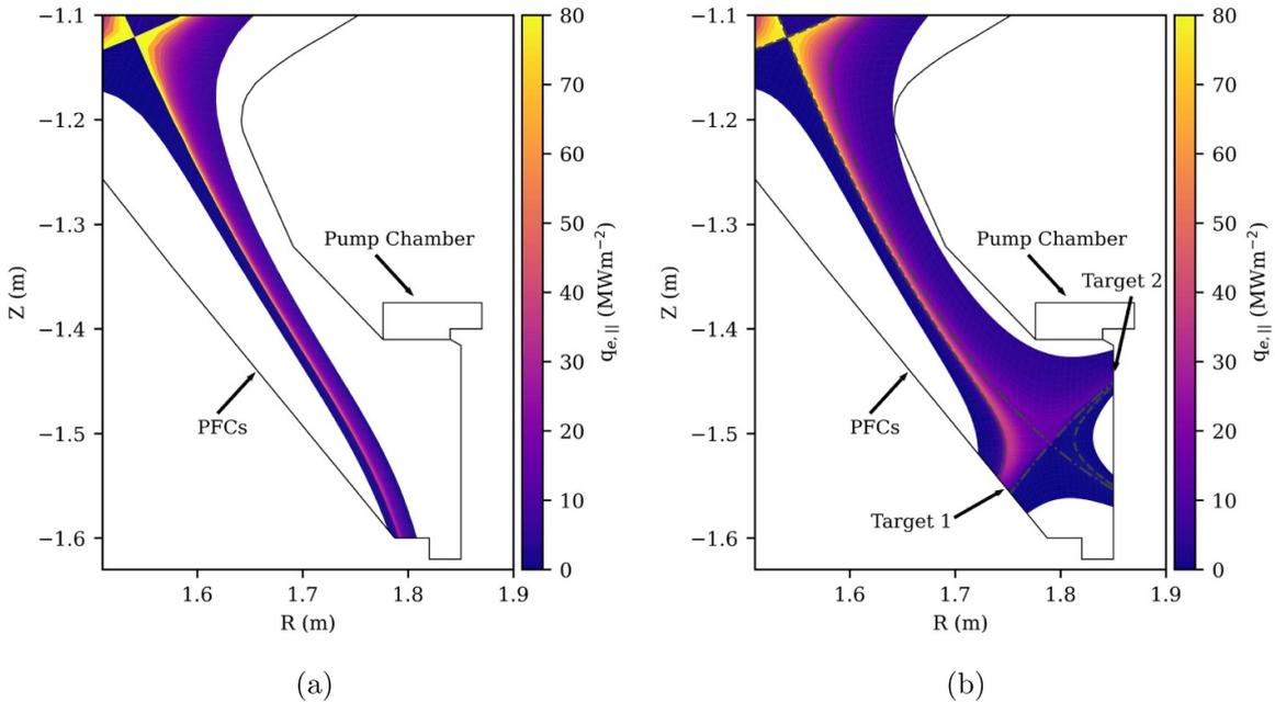
**Figure 4.** The 2D electron heat flux density profile of a (a) SPARC SN and (b) SPARC XPT SOLPS-ITER simulation. PFCs are shown in black. The two primary outer targets of the XPT are indicated, where ‘Target 1’ intersects the primary separatrix.
