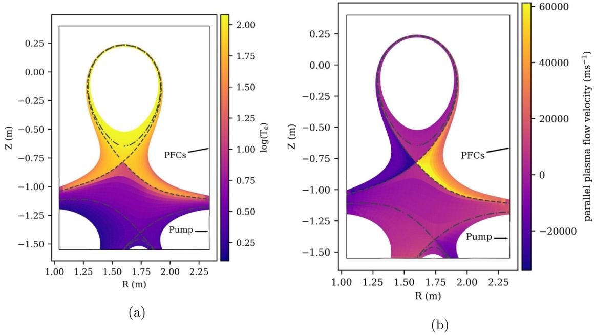
**Figure 3.** (a) A logarithmic 2d electron temperature map of a converged SOLPS-ITER simulation of a TCV-like snowflake plus equilibrium. (b) A 2d plot of plasma fluid velocity for the simulation in (a).
