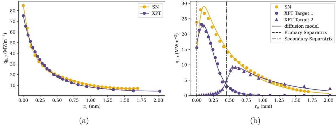
**Figure 5.** The (a) upstream and (b) target electron heat flux density profiles plotted as a function of radial distance from the separatrix (mapped to the outer midplane) for a SPARC single null and XPT divertor. Fits of the conduction-diffusion model in equation (1) are shown as unbroken lines.
