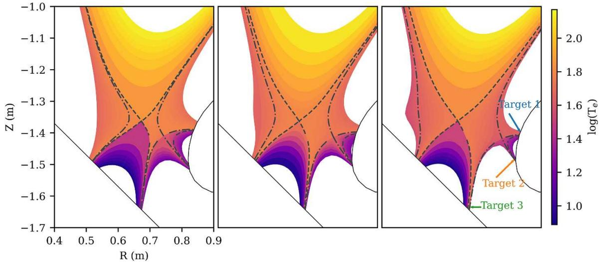
**Figure 7.** A 2d logarithmic plot of the electron temperature profiles of three MAST-U like snowflake simulations, with various X-point separations. X-point separation increases from left to right.
