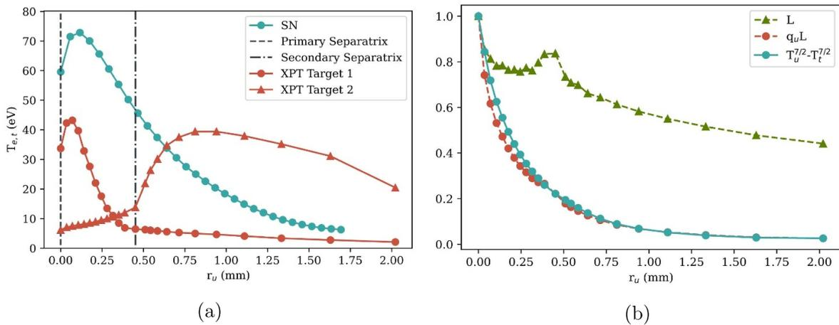
**Figure 6.** (a) The target electron temperature profiles as a function of radial distance from the separatrix (mapped to the outer midplane) for a SPARC single null and XPT divertor. (b) The profiles of connection length, product of connection length and upstream electron heat flux density, and the difference between upstream and downstream temperatures to the power  $2/7$ , plotted as a function of radial distance from the separatrix (mapped to the outer midplane) for a SPARC XPT divertor.
