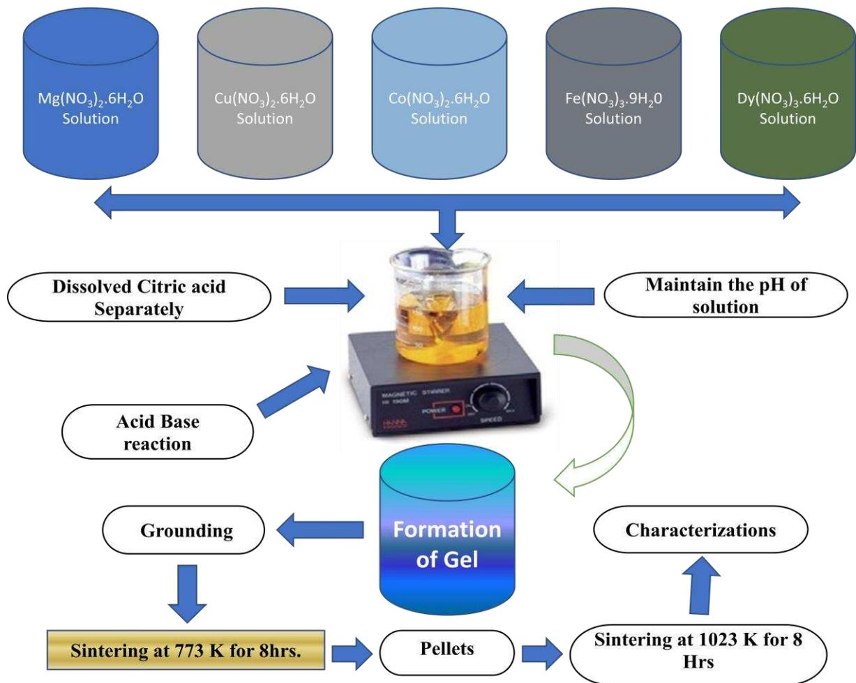
Fig. 1. Flow chart for preparation of *MCCD-soft* ferrites by sol-gel route
