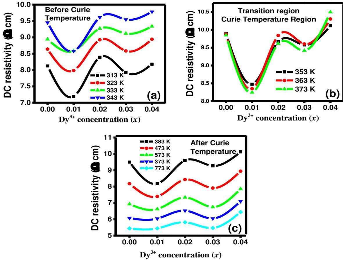
**Fig. 8.**  $\text{Dy}^{3+}$  concentration versus DC resistivity (a) before Curie temperature (b) at Curie or transition temperature region (c) after the Curie temperature for MCCD-soft ferrites
