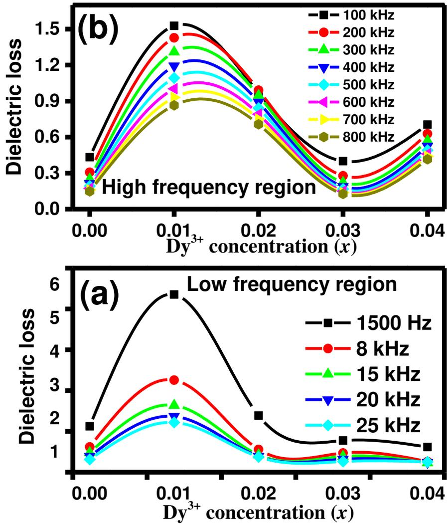
Fig. 11(a). Dy<sup>3+</sup> concentration versus dielectric loss at low frequency region (b) Dy<sup>3+</sup> concentration versus dielectric loss at high frequency region for MCCD-soft ferrites
