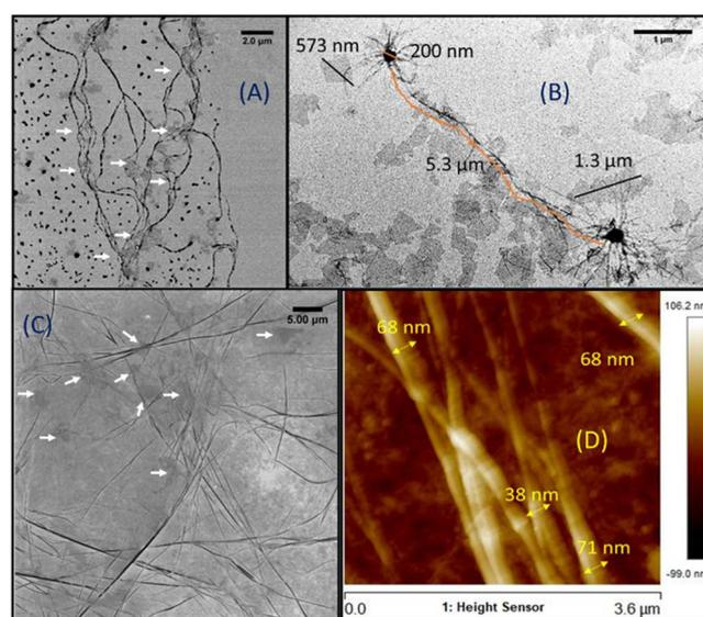
**Figure 2.** Microscopy images of the Fmoc-F/GO hybrid hydrogel. (A, C) HIM images; (B) TEM image; (D) AFM image with given dimensions of the fibers. The concentrations of Fmoc-F and GO were 2.0 and 0.25 mg/mL, respectively.
