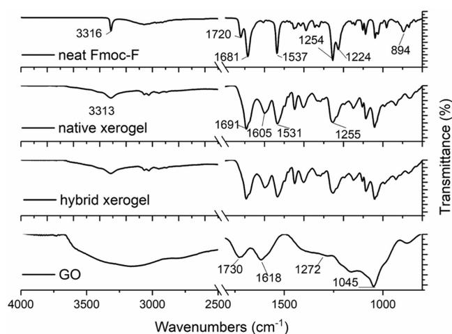
**Figure 5.** FT-IR spectra of neat Fmoc-F, neat GO, native, and hybrid xerogels. The amino acid concentration in both xerogels was 2.0 mg/mL. GO was added at a concentration of 0.25 mg/mL in the hybrid system. The FT-IR spectra of the phosphate salts  $\text{Na}_2\text{HPO}_4 \cdot 2\text{H}_2\text{O}$  and  $\text{NaH}_2\text{PO}_4 \cdot \text{H}_2\text{O}$  used for preparing PBS solution (negative control) are given in Figure S7.
