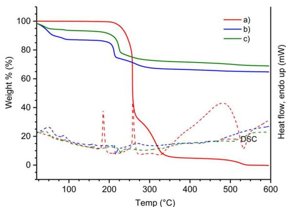
**Figure 4.** TG curves (solid lines) and DSC curves (dashed lines) of (a) neat Fmoc-F powder, (b) Fmoc-F native xerogel, and (c) Fmoc-F/GO hybrid xerogel, measured under an air atmosphere with a heating rate of 10 °C/min.
