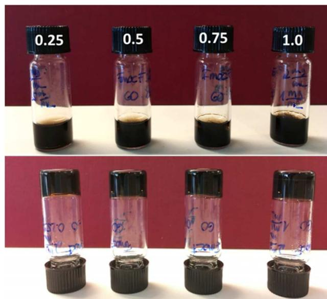
**Figure 1.** Gelation screening of the Fmoc-F/GO hybrid system at a range of GO concentrations (0.25–1.0 mg/mL). Homogeneous self-supporting gels were formed regardless of the amount of GO. The concentration of Fmoc-F was kept constant (2.0 mg/mL).
