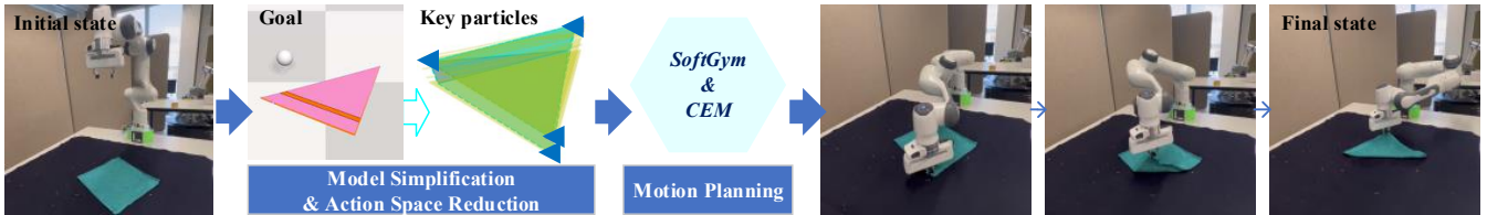
Fig. 1. Overview of the proposed approach. Given the task of folding a piece of cloth diagonally, our approach simplifies the geometric model at the goal configuration to extract the key particles as denoted by blue triangles, which represent the graspable points in the reduced action space. After that, Cross Entropy Method (CEM) is implemented to search a folding plan in the SoftGym simulator. A Franka Panda robot executes the plan in the real world and achieves a goal state.
