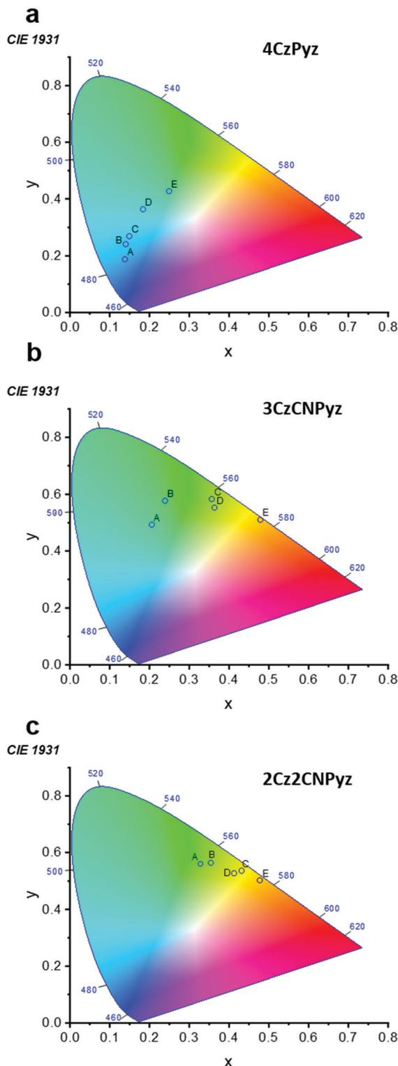
Fig. 4 The CIE 1931 curves for the photoluminescence of (a) **4CzPz**, (b) **3CzCNPyz** and (c) **2Cz2CNPyz** in a series of films. A = 0.1 wt% zeonex, B = 1 wt% zeonex, C = 10 wt% zeonex, D = 10 wt% DPEPO and E = neat film.
