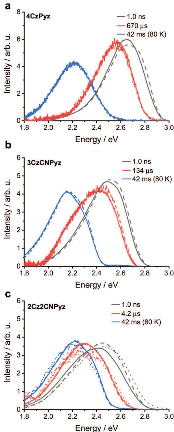
Fig. 5 The prompt and delayed emission of (a) **4CzPz**, (b) **3CzCNPyz** and (c) **2Cz2CNPyz** at 1 wt% (solid) and 0.1 wt% (dashed) in zeonex. There is also an additional 0.01 wt% concentration for **2Cz2CNPyz** represented by dotted lines.
