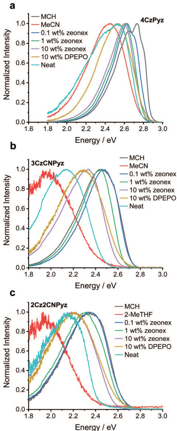
Fig. 2 The photoluminescence of 10  $\mu\text{M}$  solutions in methylcyclohexane (MCH) and acetonitrile (MeCN), doped zeonex and DPEPO films and neat films of (a) **4CzPyz** (b) **3CzCNPyz** and (c) **2Cz2CNPyz**. [N.B. For **2Cz2CNPyz** 2-MeTHF replaces MeCN as negligible signal-to-noise ratio was observed in the MeCN sample, most likely a result of severe relaxation of the CT state and associated increase in non-radiative decay].
