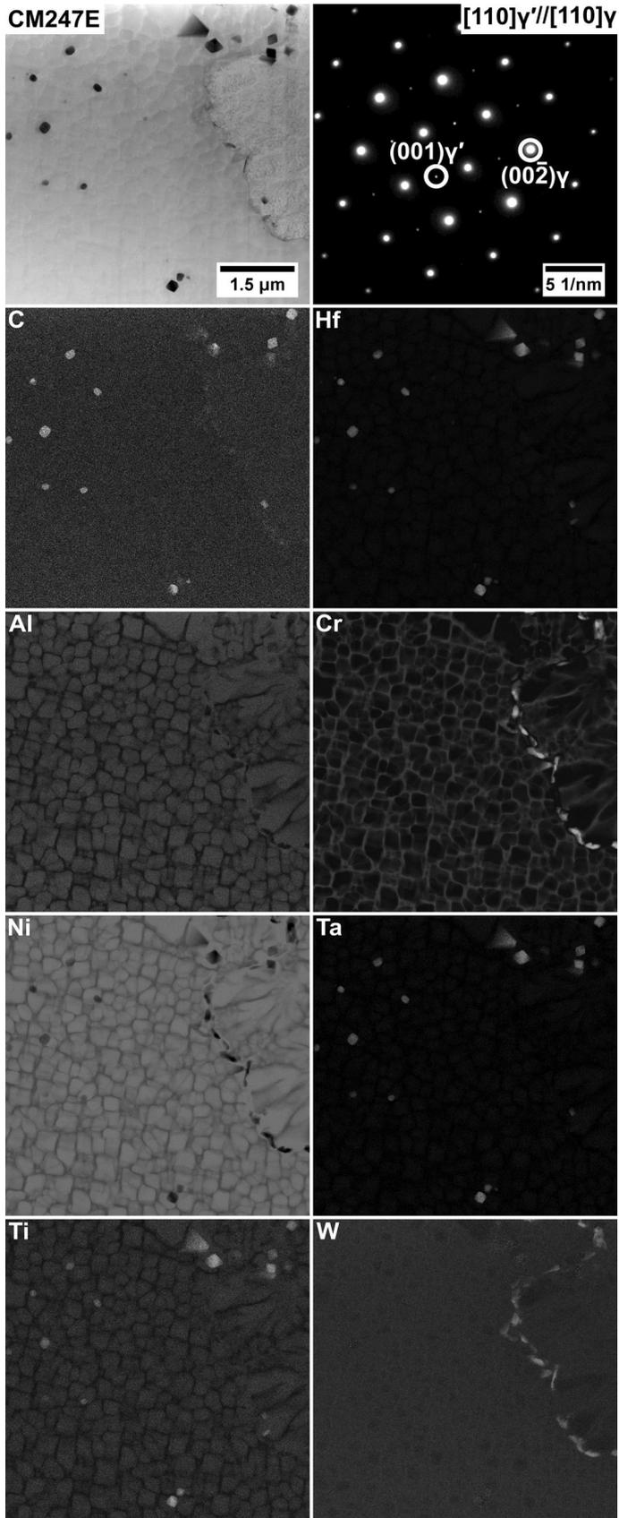
◀ Fig. 6—TEM analysis of L-PBF CM247LC in the heat treatment E condition. A bright field electron image is shown at the top left; accompanied by a selected-area electron diffraction pattern for the matrix along [110] at the top right. Below are elemental distribution maps determined by STEM-EDX.
