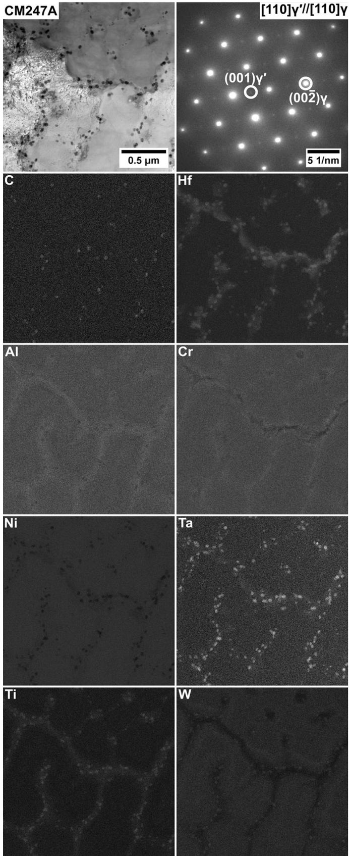
◀Fig. 5—TEM analysis of L-PBF CM247LC in the heat treatment A condition. A bright field electron image is shown at the top left; accompanied by a selected-area electron diffraction pattern for the matrix [110] at the top right in which specific reflections from the  $\gamma$  and  $\gamma'$  phases are identified. Below are elemental distribution maps determined by STEM-EDX.
