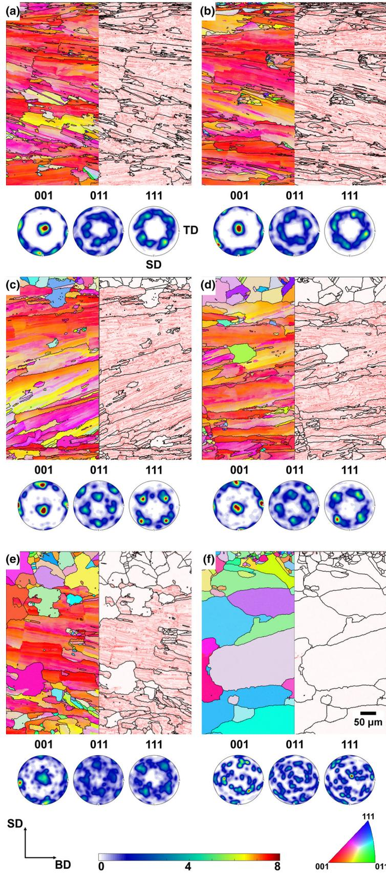
◀ Fig. 8—SEM-EBSD analysis of L-PBF CM247LC specimens in post-processing conditions (a to f). These conditions are detailed in Table II. Samples were taken from the centre of each build, with an edge region visible. For each sample an IPF map oriented along the build direction has been stitched with the corresponding KAM map. In addition, cubic pole figures oriented down the build direction have been provided for each sample below the maps.
