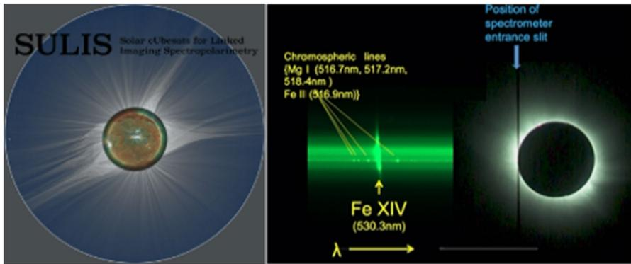
**Fig. 4** *Left:* The spectro-polarimeter (occluding CubeSat) will observe the solar disc and inner atmosphere. The coronagraph (coronagraph CubeSat) will observe extended coronal structures and CMEs. *Right:* Example of the spectrometer eclipse measurements. The slitjaw image on the right shows the slit position, the high-resolution spectra are on the left
