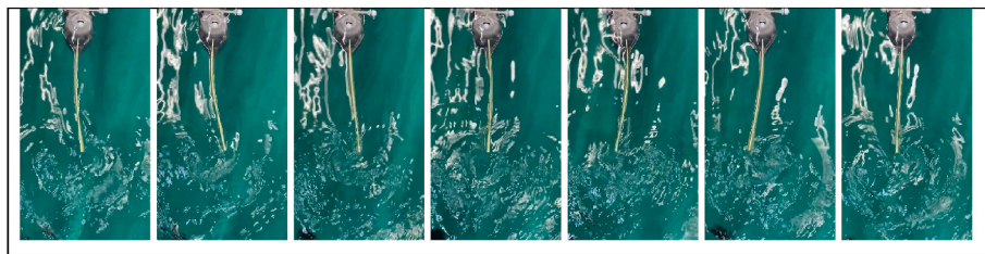
Fig. 19. Elastic displacement of Foamex tail plate.
