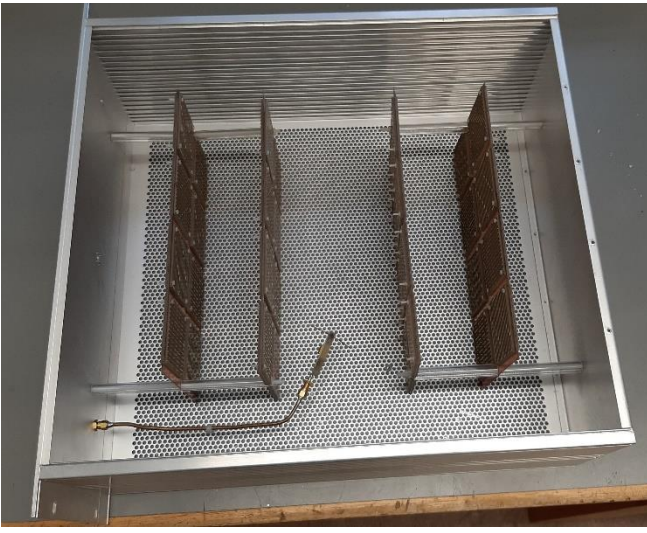
Fig. 5. Image of the simulated EUT showing circuit cards and the internal dipole antenna situated between the resistively loaded circuit cards.
