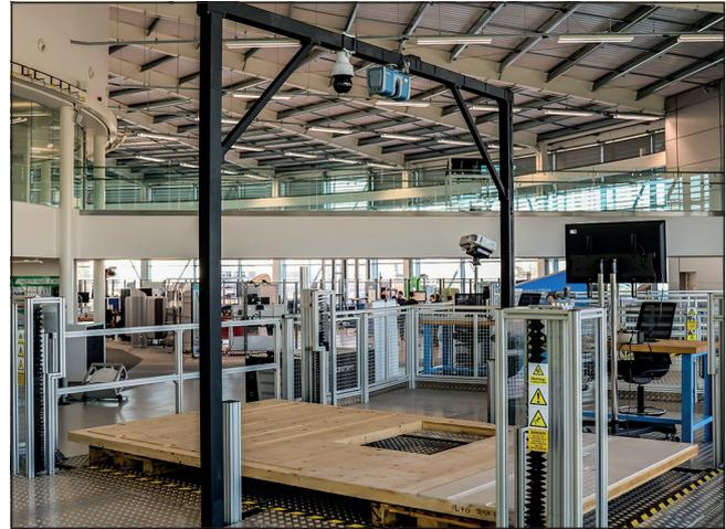
Figure 7. Inspection cell for checking a CLT wall panel using a 3D laser scanner
