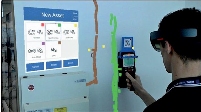
Figure 5. An example of data capture with a Microsoft HoloLens headset and a Bosch D-Tect handheld wall scanner
