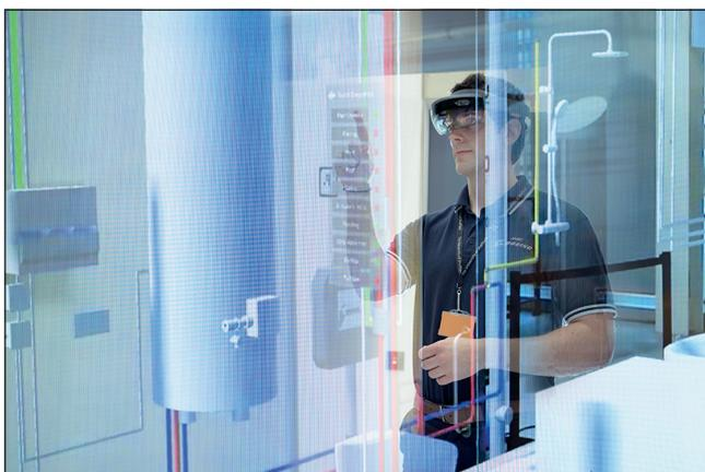
Figure 2. Microsoft HoloLens headsets allow users to see a virtual overlay on a physical asset
