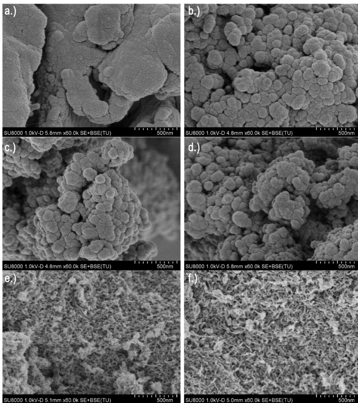
Fig. 1. SEM of a.) alginate acid, b.) expanded alginate acid (A90), c.) A300, d.) A450, e.) A600 and f.) A800. Conditions: SU8000 Hitachi SEM, 1.0 kV-D ~5.0 mm.
