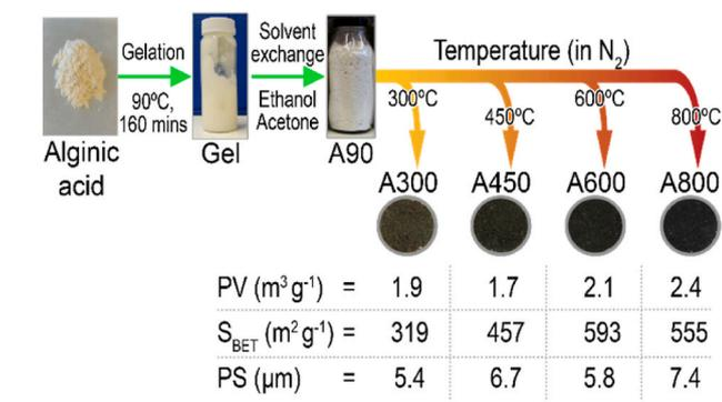
**Scheme 1.** Schematic of the synthetic route to prepare the alginic acid derived mesoporous carbonaceous materials, A300, A450, A600 and A800, where PV = pore volume,  $S_{\text{BET}}$  = BET surface area, and PS = particle size.
