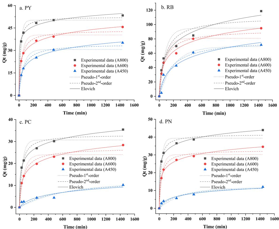
**Fig. 3.** Kinetic data fittings on the initial stages of dye adsorption using the adsorbents A450, A600 and A800, where a.) PY b.) RB, c.) PC and d.) PN. Conditions: dye solution volume 100 mL; concentration 65 mg/L for PY, 31 mg/L for RB, 46 mg/L for PC, 61 mg/L for PN; pH neutral; temperature 25 °C; stirring rate 200 rpm; adsorbent dosage for RB 20 mg, for PY, PC and PN 100 mg.
